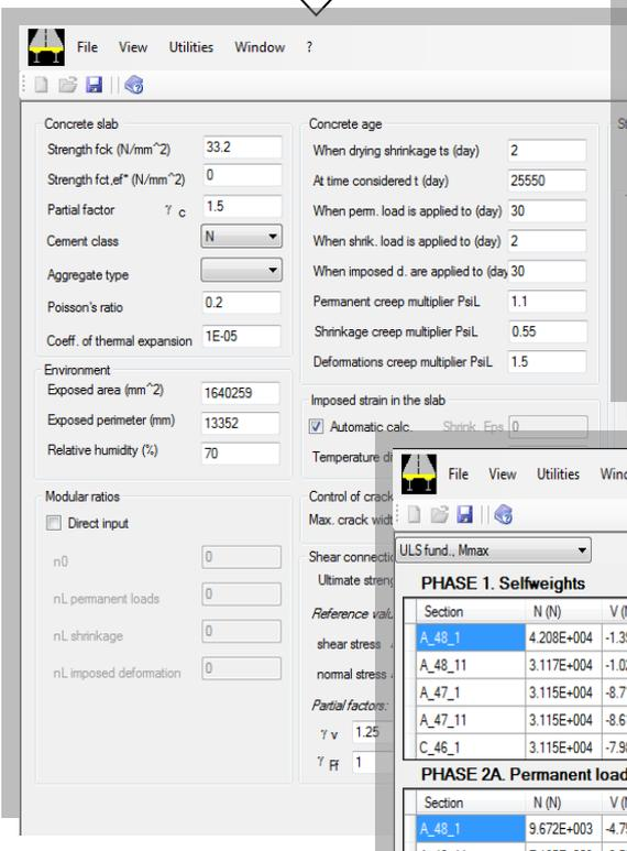
Load effects for the various sections to be checked are entered in a spreadsheet style. Construction stages and in-service conditions are assimilated and design combinations organised in groups
