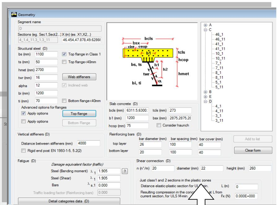
Sections are described by the engineer in a simple dialog box and organized in a tree structure
